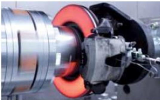
At the performance test at the test bench, the friction coefficient and the brake pad’s bedding-in at different pressures are measured thus simulating years of use in vehicles.
