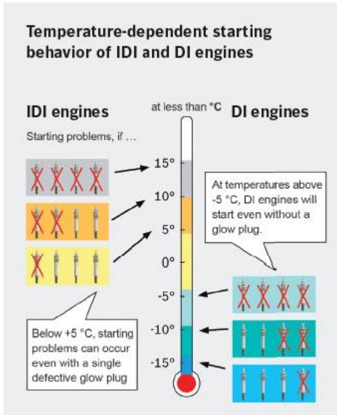
The starting behavior of IDI and DI engines very much depends on the temperature. Especially in case of defective glow plugs during the cold season, this leads to starting problems. With one defective glow plug, IDI engines will experience starting problems already at 5 °C. Customers should thus be informed about this topic actively and on time.
