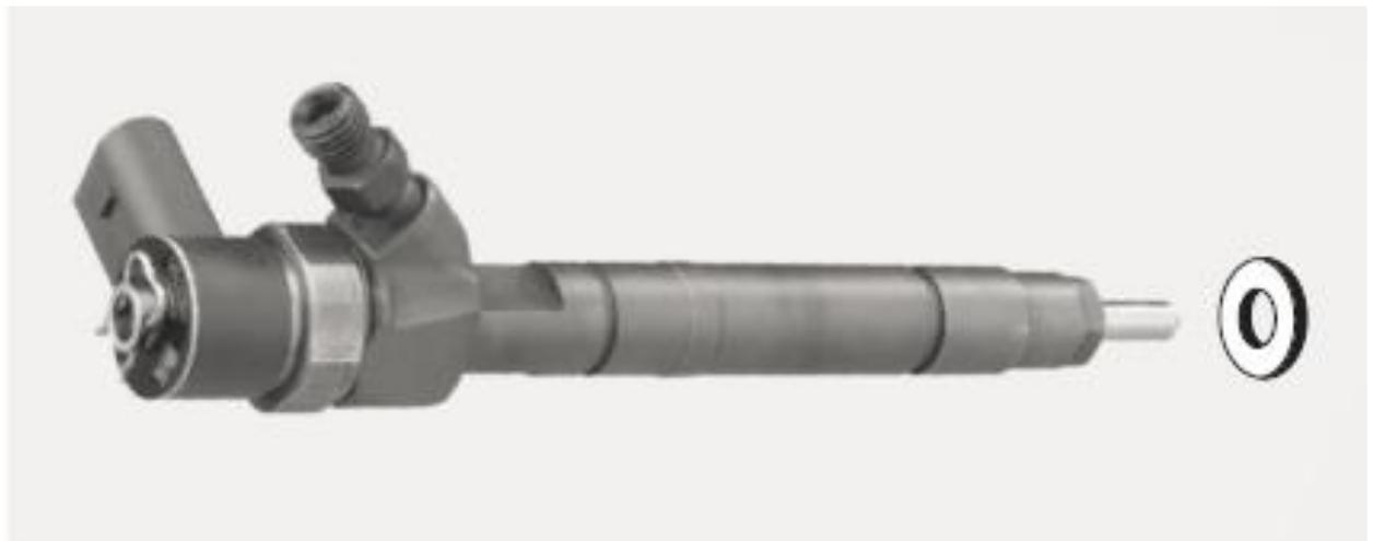
The CR injector is usually supplied with a seal. To ensure proper engine operation it is essential to compare the thickness of the original seal to that of the new seal provided (dimension "s" in table on Page 2).
