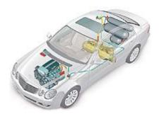
Bivalent vehicles have two tanks and can run on both natural gas and gasoline. In other words, switching is possible at any time from gas to gasoline operation – convenient switching from
