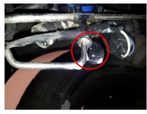
Within the red marking, foam formation can be seen at the gas pipe. This is an indication of leakage.
