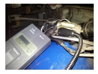
The display shows leakage at the connection.
