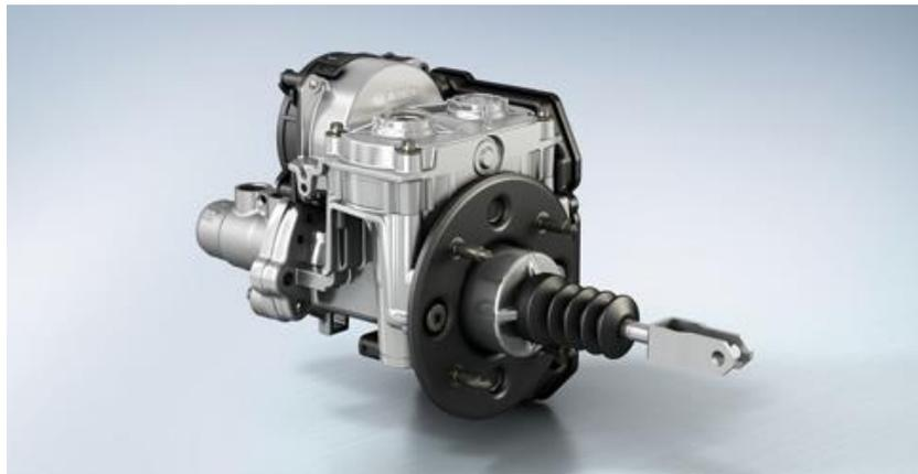
The iBooster by Bosch therefore satisfies an important requirement of automated driving. The braking force amplifier can build up to braking pressure independently and three times faster than an ESP®-System. If for example the predictive emergency braking system identifies a hazardous situation, the vehicle comes to a stop much faster. At the same time, the iBooster also handles the smooth braking of adaptive cruise control ACC up to a standstill almost entirely noise-free.
