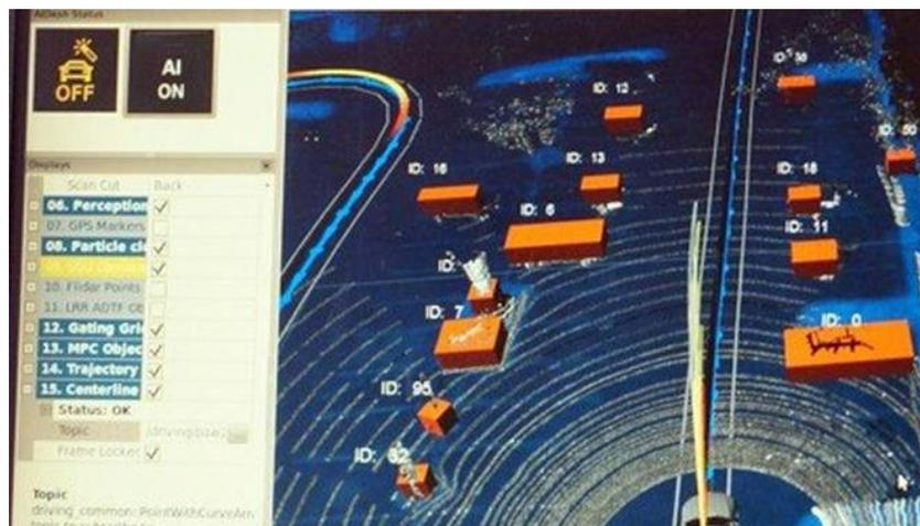
The data from the individual sensors are compiled and converted into a comprehensive model of the surroundings. All static and dynamic objects are depicted. Entirely new hardware and software technologies and algorithms are used in these calculations. Then the identified objects are placed in a precise relationship to traffic lanes, and the vehicle is located on digital maps. The automated driving system can interpret the situation, identify unrestricted routes and to develop a driving strategy.
