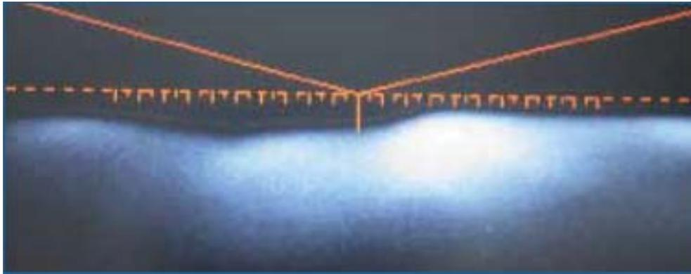
Vehicles with light assistance functions exhibit distinctly different shapes for the light-dark boundary from one manufacturer to another. For this reason, intelligent lighting systems have a specific setting mode for evaluating the light-dark boundary. The manufacturer provides reference values for this purpose.
