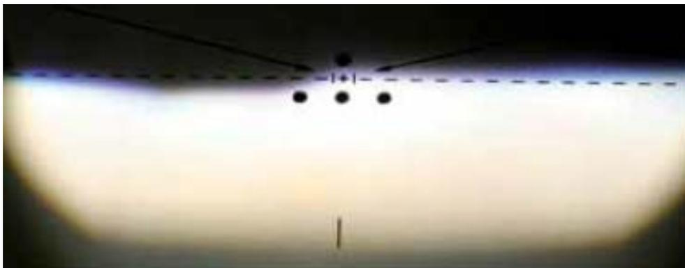
Because of the blue fringe of the xenon light, the eye is not able to detect the exact light-dark boundary clearly. The exact evaluation and adjustment of headlamps required for safe traffic cannot be achieved with an analog headlamp beam setter.
